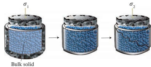
Fig. 10 Steps of the uniaxial compression test. The first step (left) is the consolidation of particles inside the cylinder under a normal stress \sigma_1 . In the next step, we remove the cylinder. At the final step (right), the particles will experience a failure at a certain stress \sigma_2 called unconfined yield strength.
