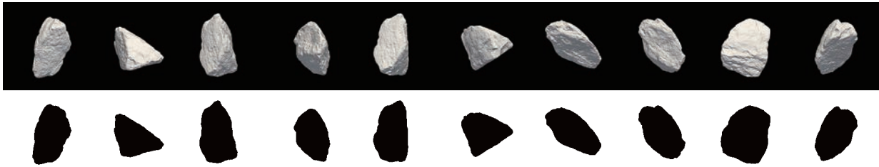
Fig. 10 Ten 2D projection images of a VG-A particle.
