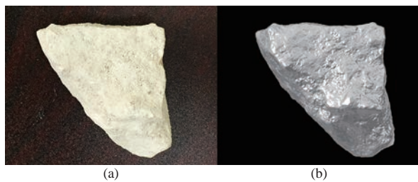
Fig. 5 Captured 3D particle geometry using 3D SL scanning: (a) original particle; and (b) digitally represented particle (Bhattacharya et al., 2020); image reused with written permission from the publisher.
