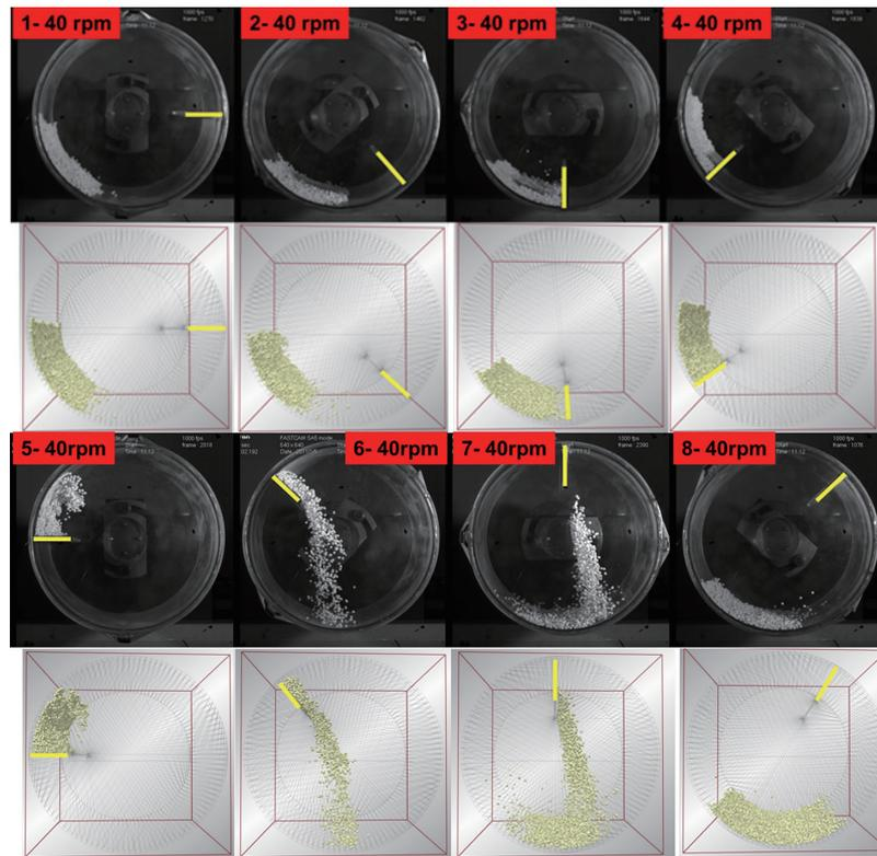
**Fig. 6** An example of the use of optical data for the validation of DEM simulations for a laboratory-scale rotating drum. Image reproduced from Ref. (Marigo and Stitt, 2015) under the terms of the CC-BY 4.0 license. Copyright: (2015) The Authors, published by Hosokawa Powder Technology Foundation.
