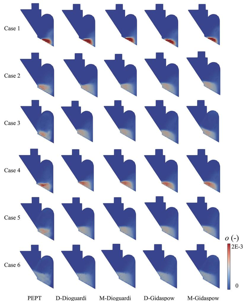
**Fig. 8** Comparison of PEPT and CFD–DEM derived solid occupancy distributions for a variety of different system conditions (rows) and drag models (columns). Reproduced with permission from Ref. (Che et al., 2023a). Copyright: (2023) Elsevier B.V.
