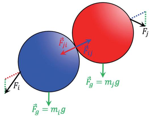
**Fig. 1** A schematic illustration of two interacting DEM particles. Particle  $i$  is subject to a gravitational force  $\vec{F}_g$  proportional to its mass  $m_i$ , and a contact force  $F_{ji}$  due to contact with a second particle  $j$ . The net force  $F_i$  acting on the particle is used to predict its position and velocity at the next point in time. Reproduced with permission from (Rosato and Windows-Yule, 2020).
