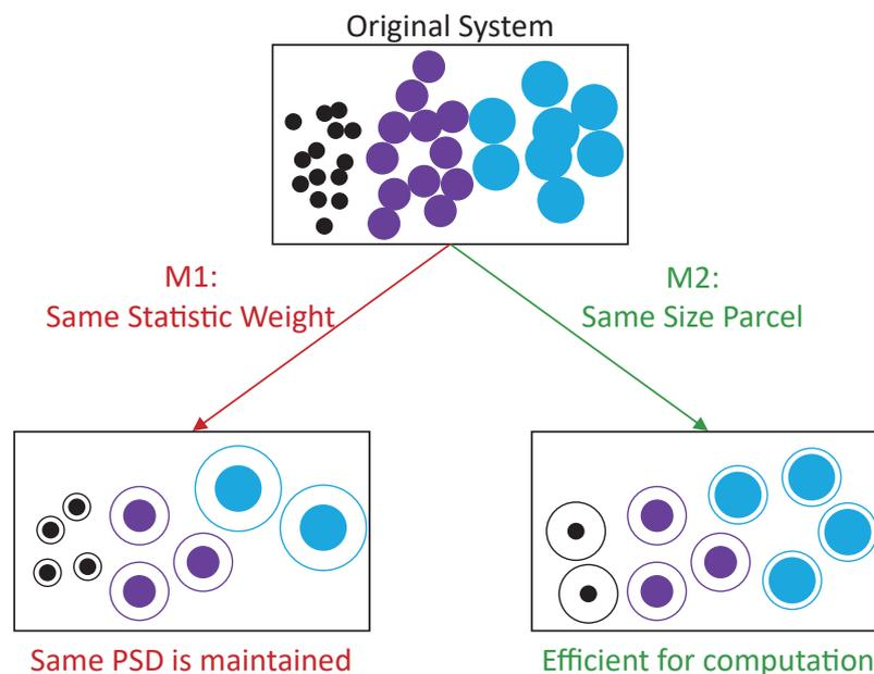
**Fig. 4** Simple schematic depicting the two methods for the coarse-graining of polydisperse systems described in the main text. Adapted with permission from Ref. (Lu et al., 2018). Copyright: (2018) Elsevier Ltd.
