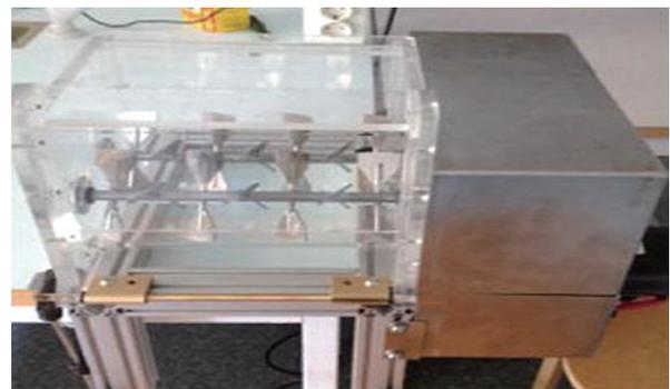
**Fig. 9** Image of the 2 L paddle mixer, reprinted with permission from Ref. (Shenoy et al., 2015). Copyright: (2015) Elsevier B.V.
