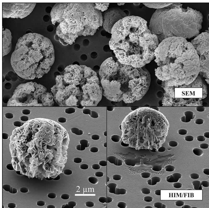
**Fig. 11** Scanning electron microscopy (SEM) and helium ion microscopy (HIM) micrographs of leucine particles collected from a monodisperse droplet chain instrument (Ordoubadi et al., 2019). The particle at the bottom was also cut using focused ion beam (FIB) milling to study the interior morphology. All micrographs are reproduced with the permission of Springer Publishing.
