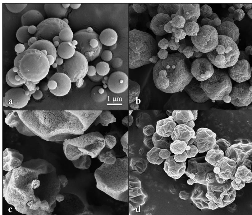
**Fig. 4** Micrographs of spray-dried trehalose and different shell formers: (a) trehalose; (b) trehalose and 20 % w/w L-leucine; (c) trehalose and 5 % w/w trileucine; (d) trehalose and 3 % w/w Eudragit. (Reproduced from Bin Karim et al., 2021 with the permission of Elsevier.)
