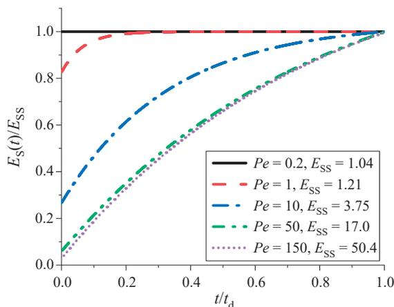
**Fig. 6** The time evolution of surface enrichment,  $E_s(t)$ , normalized by the steady-state surface enrichment,  $E_{ss}$  (Eqn. (6)), versus the normalized time for different Péclet numbers, obtained from the correlations given in Eqn. (7). Here,  $t_d = d_0^2 / \kappa$  is the droplet drying time.
