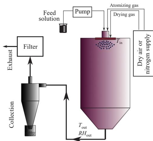
**Fig. 1** A typical open-cycle spray dryer showing the key stages of atomization, drying, and collection.
