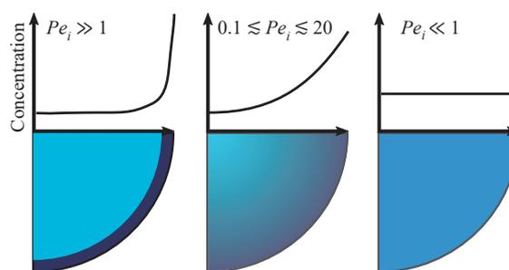
Fig. 5 The effect of the Péclet number on the internal solute distribution during droplet evaporation at a specific time.
