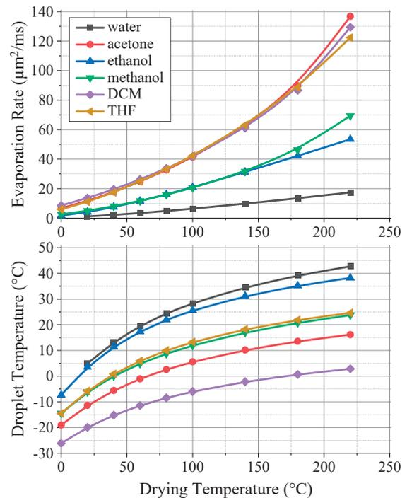
**Fig. 7** The evaporation rates and droplet temperatures of several solvents frequently used in pharmaceutical spray drying at different drying temperatures. The values were calculated using a full numerical model.
