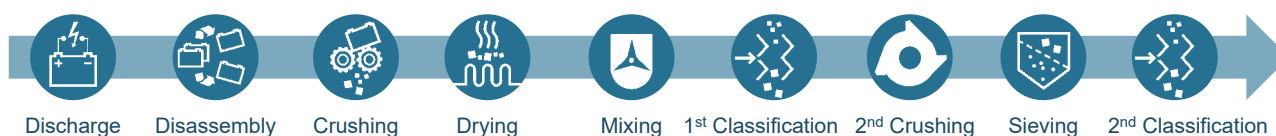
Fig. 4 Exemplary process diagram for the LithoRec recycling process for LIB. Reprinted with permission from Ref. (Kwade and Diekmann, 2018). Copyright: (2018) Springer Nature.
