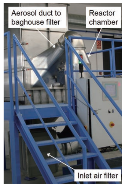
Fig. 7 Fully enclosed FSP pilot plant at Tecan (Los Arcos, Spain): The cooling air inlet is equipped with a filter to purify the air and to prevent the release of nanoparticles in the case of an aerosol backflow. The nanoparticle-producing spray flame is located inside the reactor chamber that is directly connected to the baghouse filter, minimizing the aerosol volume.
