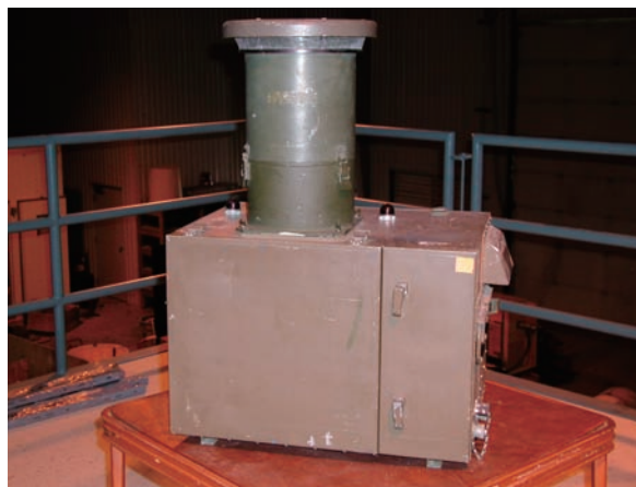
Fig. 2 XM19 biological detector showing the virtual impactor stack.
