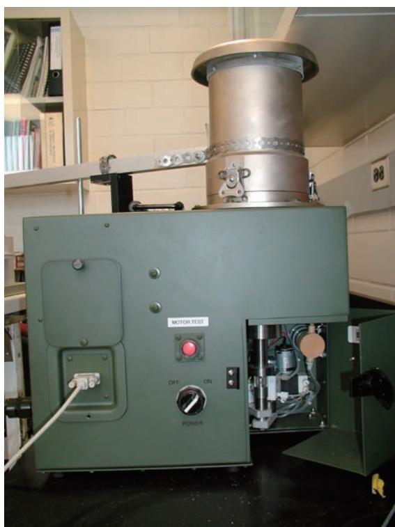
Fig. 8 A commercially available virtual impactor that can be configured to collect aerosol particles in sequential 1-2 ml liquid fractions. Conventional 96 well plates may be used to archive the time stamped samples. The instrument can also be configured for single liquid tube or a dry filter collector (Dycor Technologies Ltd, Edmonton, Alberta, Canada).
