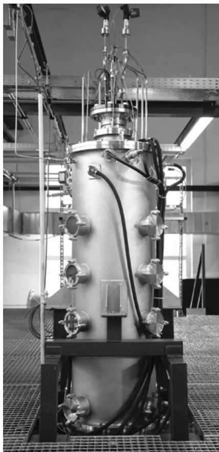
Fig. 2 Hot-wall reactor mounted in the pilot plant. Several ports allow for optical in-situ diagnostics in the hot reaction zone with nozzle on top of the reactor.
