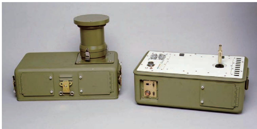
Fig. 6 Prototype FLAPS3 showing a virtual impactor on the left and the particle detection electronics on the right. The coupling of the two systems was accomplished via a spring loaded aerosol transfer tube shown as a golden extension on the right unit. Combining the two units with four clasps resulted in a single one person portable instrument that was designed to be weather proof. In practice, it performed well during a tropical storm. Consequently, it was possible to sample biological aerosol content during rainy periods. This capability opened up a hitherto unprecedented opportunity to explore the presence of biological aerosol content associated with rain episodes.
