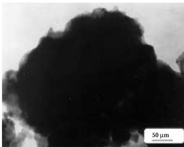
**Fig. 15** Microphotograph of a  $\text{BaZrO}_3$  particle obtained by mechanochemical synthesis during 1 minute.
