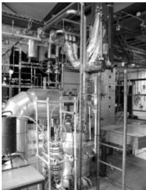
**Fig. 5** Low-Pressure Flame Reactor.
