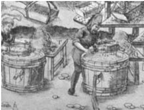
**Fig. 1** Settling tanks described by Agricola (1556).
