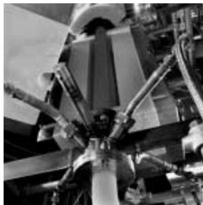
**Fig. 9** Photograph of the pilot-scale hot-wall reactor operated by the Project House Nanomaterials.
