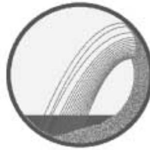
**Fig. 11** Simulated Charge Profile Corresponding to a Lifter Bar of 120 mm and Angle of  $90^\circ$  for a 9.6 m diameter SAG mill.
