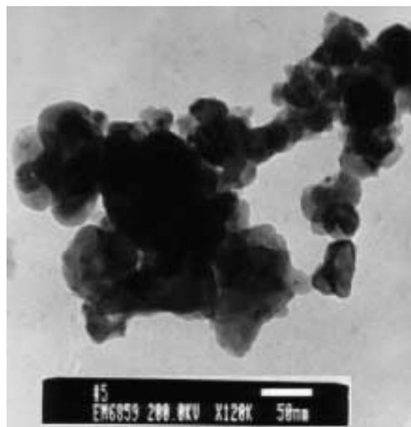
**Fig. 21** Microphotograph of the product of mechanochemical interaction of  $\text{BaO}_2 + \text{WO}_3$  (time of MA 5 min.).
