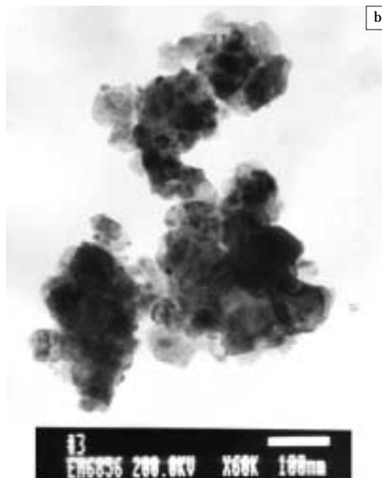
**Fig. 18** Microphotograph of the SHS product of a  $\text{BaO}_2 + \text{WO}_2$  mixture (a), the same product after mechanical activation for 2 min. (b).
