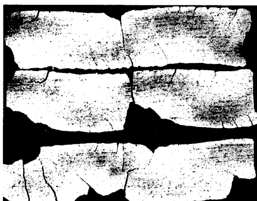
Fig. 11 Strip of a mix (monohydrate lactose+0.5% magnesium stearate+5% [200-400 \mu\text{m} ] coal particles) compacted with a screw speed of 7.7 rpm and a roller speed of 2.2 rpm. Rolling is from left to right.
