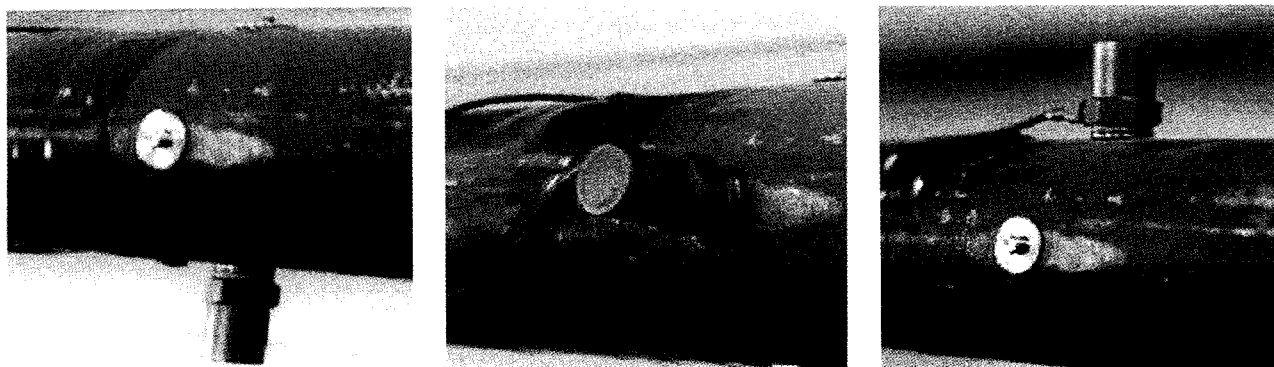
Fig. 5 Details of accelerometer mounting (from left to right): bottom mounting – side mounting – top mounting. Note that it is imperative to affix cabling firmly to pipeline surface to ensure that the cabling receives the same vibrations as the accelerometer bracket(s). Also note bracket preparations on pipeline surface.
