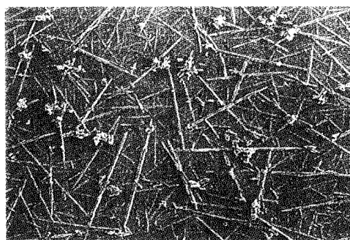
Fig. 8 Particles of the Drug Levostatin Formed with the RESS Method (extraction temperature: 55°C; extraction pressure: 200-250 bar; preliminary expansion temperature: 100-110°C)
