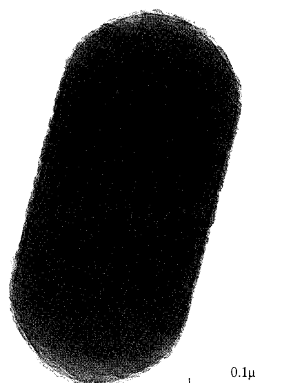
Fig. 2 Electron micrograph of a silica coated rutile prepared by the dense silica method. The coherent nature of the coating is demonstrated.
