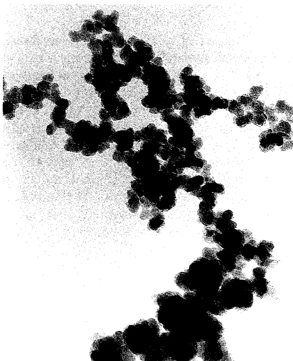
Fig. 7 TEM photograph of agglomerated \text{Si}_3\text{N}_4 particles
