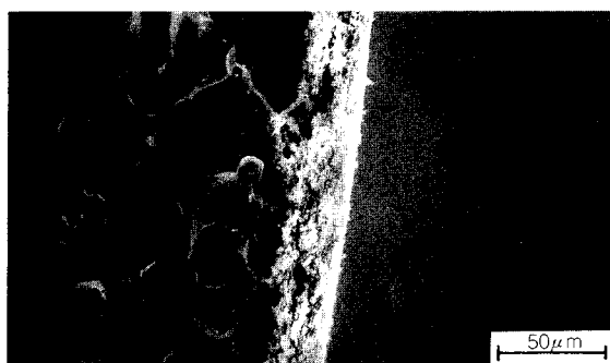
Fig. 7 Sectional photograph (SEM) of the ceramic membrane
