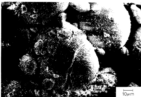
Fig. 15 Coating of the core particles using agglomerated guest particles
