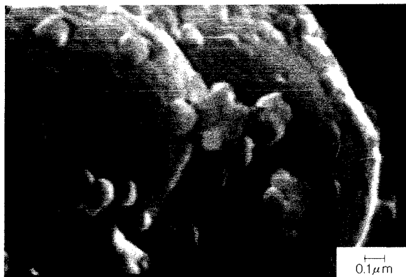
Fig. 13 Guest particles embedded in the core particle surfaces
