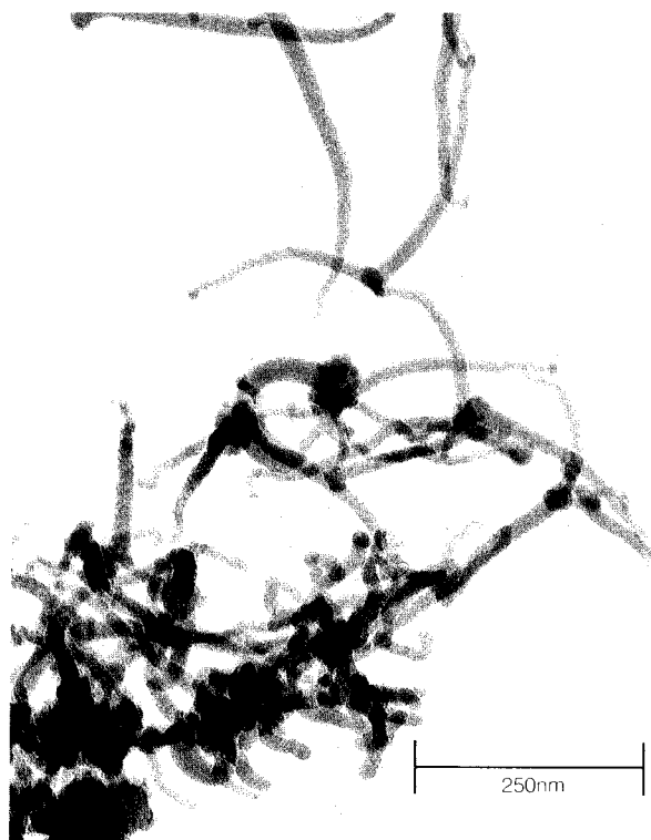
Fig. 9 TEM photograph of amorphous fibers from \text{NH}_3 and \text{SiH}_2\text{Cl}_2
