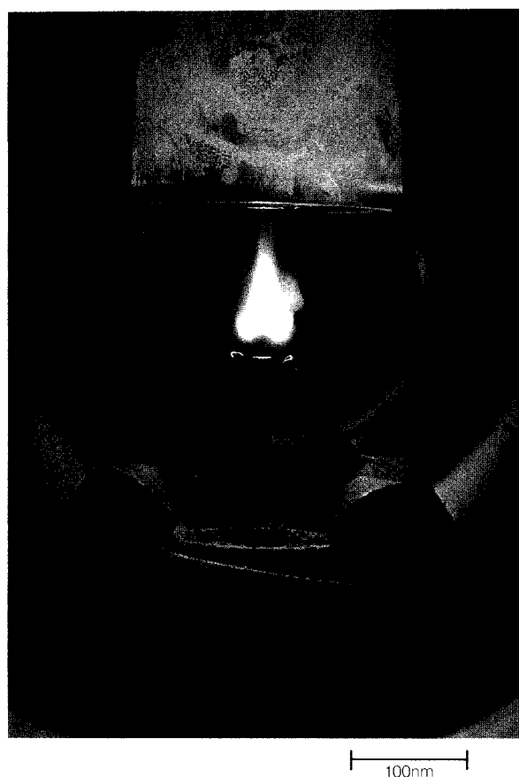
Fig. 3 Laser reaction flame produced by excitation of \text{SiH}_2\text{Cl}_2
