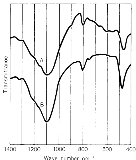
Fig. 3 IR spectra of rice hulls which was heated in 1N \text{HNO}_3 solution or under reduced pressure
