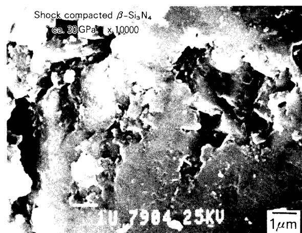
Fig. 9 SEM of explosively shocked \text{Si}_3\text{N}_4 ( \beta - \text{Si}_3\text{N}_4 , ca. 30 GPa)
