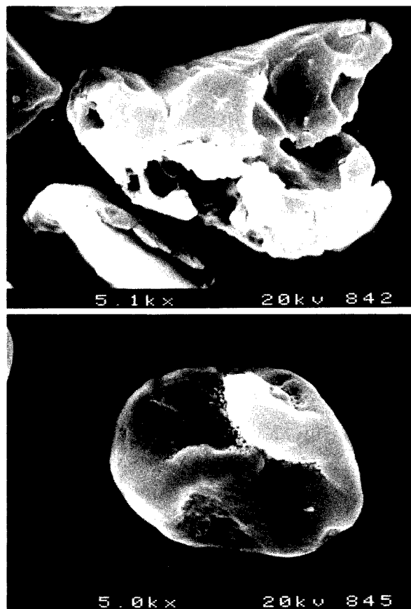
Photo 7 upper : Ground polystyrene resin lower : Particle treated with carbon black.
