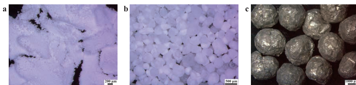
Fig. 1 SM images of the raw materials: a , La 2 O 3 , b , B 2 O 3 and c , Ca.
