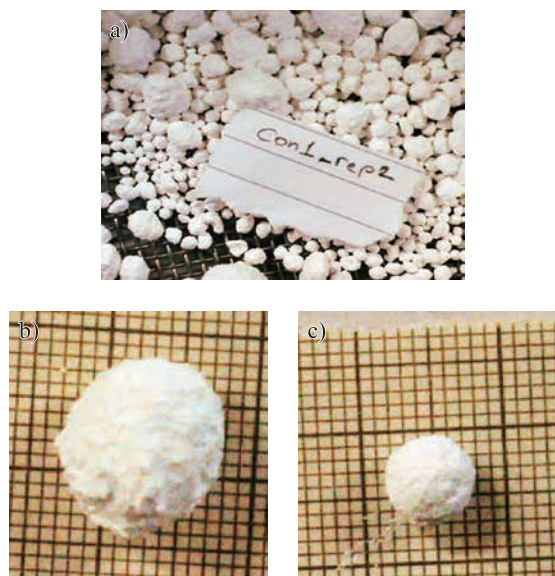
Fig. 3 Examples of agglomerates formed: a) 2-mm oversize fraction for CaCO 3 ; b) CaCO 3 ; c) TiO 2 .
