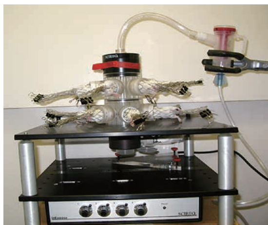
Fig. 3 InExpose TM (SCIREQ ® ) nose-only exposure system.
