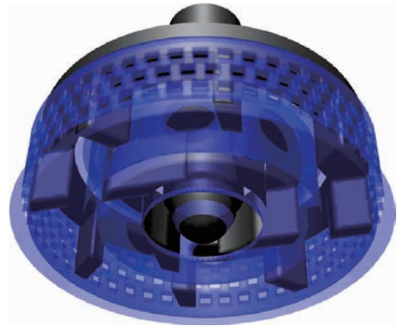
Fig. 18 Rotor-stator computational grid showing device geometry.
