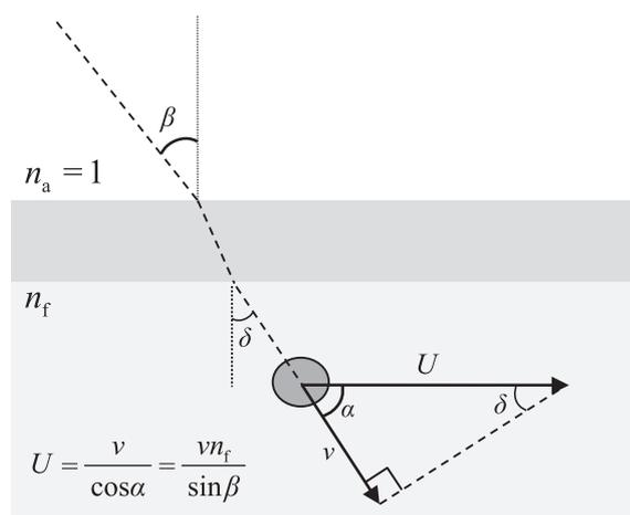
**Fig. 3 c)** A closer look at the measurement optics. Here  $U$  is the real velocity,  $v$  is the component of velocity in the direction of the measurement beam, and  $n_f$  is the refractive index of the medium. Angle  $\alpha$  is obtained by calculating first angle  $\delta$  by applying the Snell's law of refraction to the two interfaces.
