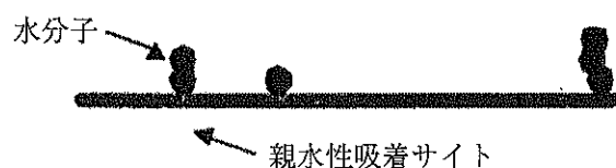
Fig. 4 Model of multilayer adsorption of water vapor on hydrophobic surface
