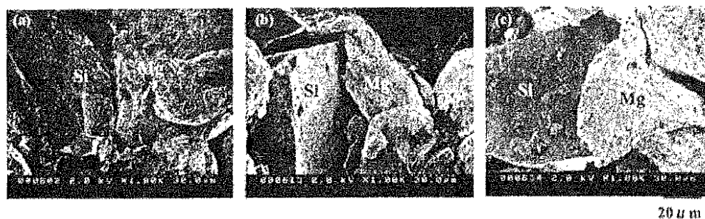
Fig.2 SEM observation on Mg-33.33mol%Si green compact consolidated at 100MPa (a), 300MPa (b) and 600MPa (c).
