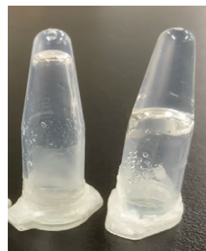
Fig. 3 Photographs of gels formed after mixing Alb-SPDP solution with PEG derivative ( Left ; 2.5% Alb-SPDP solution, Right ; 5% Alb-SPDP solution).
