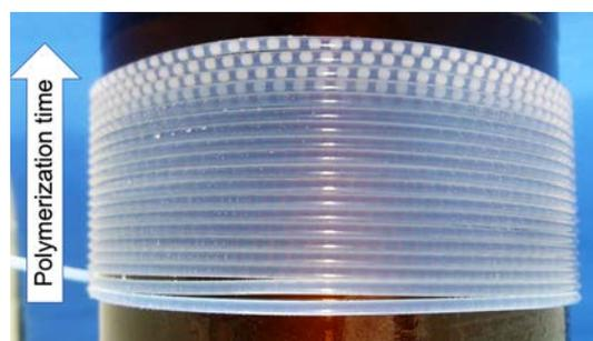
Fig. 2 Image of a reaction tube immersed in an oil bath. The reaction proceeded from the bottom to the top of the image.
