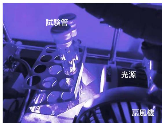
**Fig. 1** Reaction set-up for photo-catalytic decarboxylative alkylation of carboxylic acids with electron-deficient alkenes.
