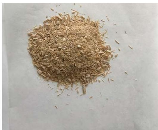
Fig. 1 Photo of bamboo powder used in this study.
