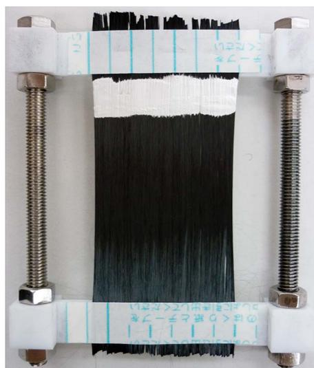
Fig. 1 Appearance of unidirectional SiC fiber preform.
