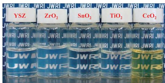
Fig. 3 Dispersion behavior of ceramics nanocrystals in water.
