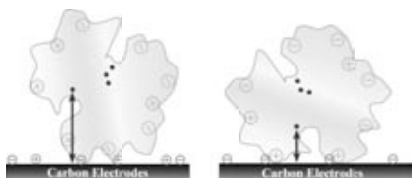
Fig.10 Adsorption image of BOD by the electrostatic interaction between BOD and the carbon electrode surface.
