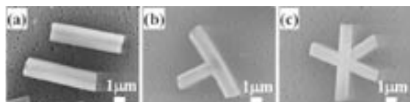
Fig.1 Typical SEM images of multibranch C 60 fine crystals. The concentration of C 60 solution is the 1 mM. (a) shows images of nonbranched C 60 fine crystals, i.e., rodlike C 60 fine crystals, for reference.
