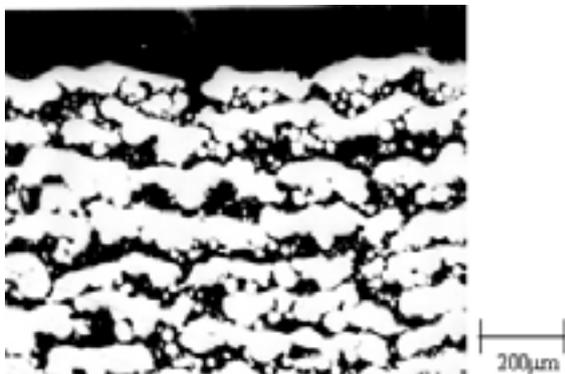
Fig.12 Sectional view of the multi-layered compact in vacuum sintering.
