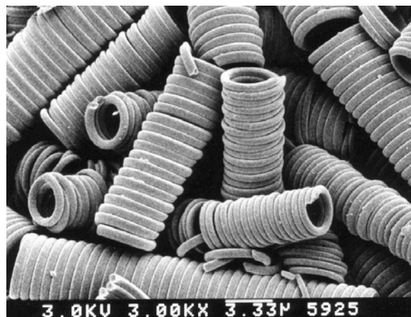
Fig. 2 Pulverized CMCs (CMC powder) .
