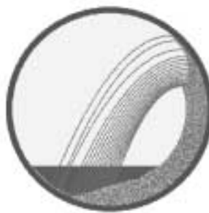
Fig. 11 Simulated Charge Profile Corresponding to a Lifter Bar of 120 mm and Angle of 90° for a 9.6 m diameter SAG mill.
